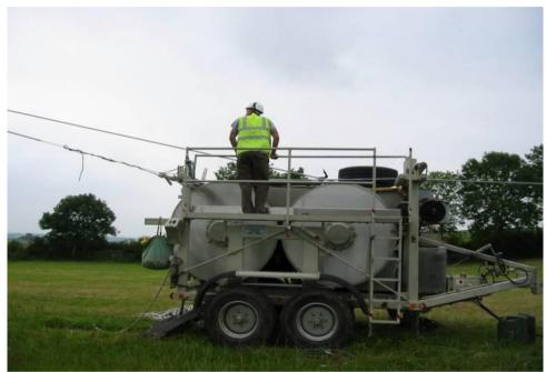
Figure 7.1: Puller – Tensioner machine
